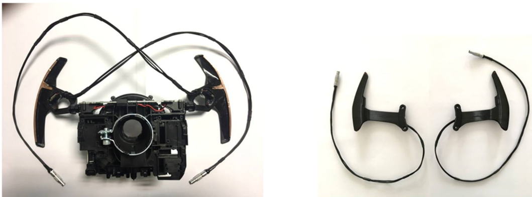
Prototype paddle shifters with touch-sensitive surfaces for driving simulator
